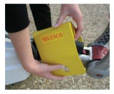
1. Ensure stabiliser red handle is in upright position and the black handle is in the down position.
