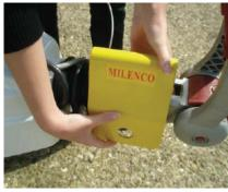
2. Place the body of hitch lock over the black handle ensuring it is located into the slot in the inside top corner of the hitch lock.
