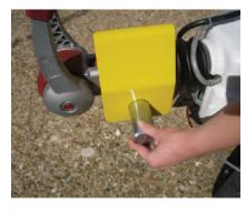
3. Place the bolt through the hole on the hitch lock body
